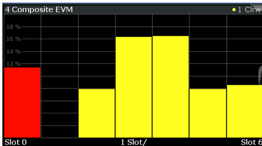
Fig. 3-5: Composite EVM display for TD-SCDMA BTS measurements
