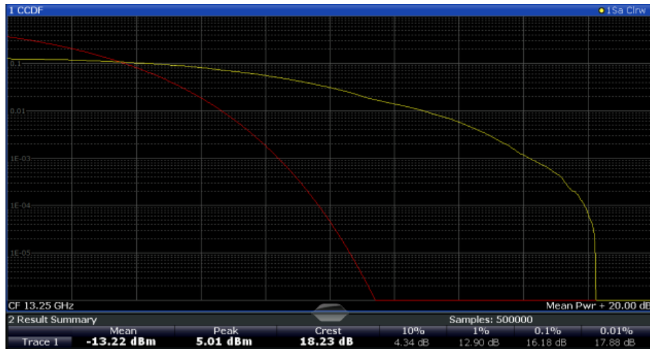
Fig. 3-22: CCDF measurement results for TD-SCDMA BTS measurements
