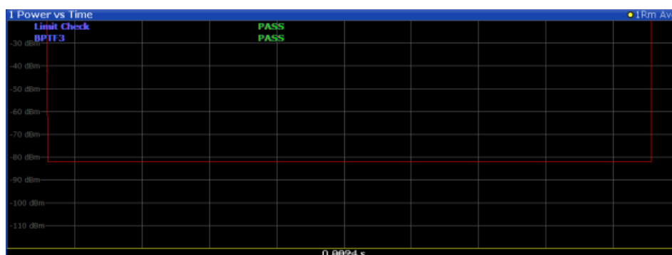
Fig. 3-16: Power vs Time diagram for TD-SCDMA BTS application
